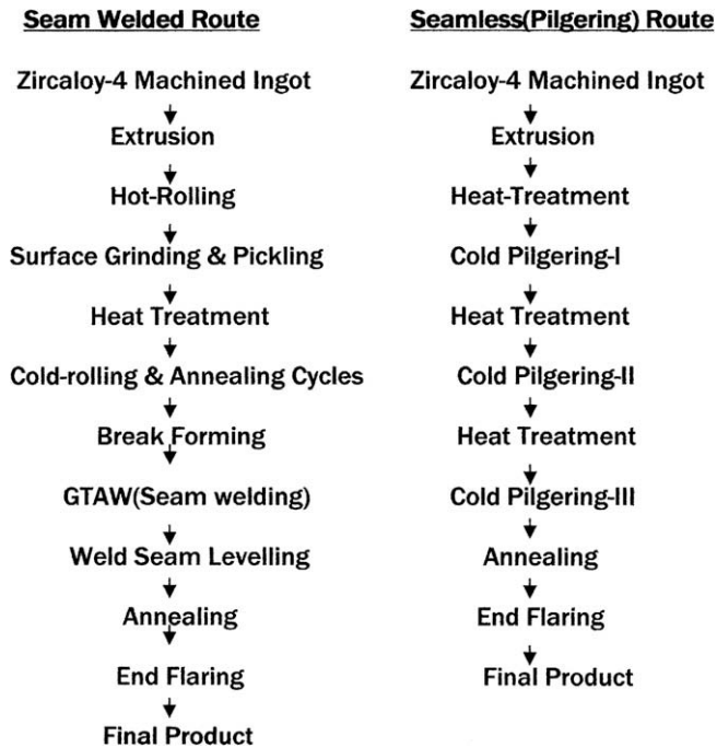
Fig. 1. Fabrication routes for calandria tubes.
